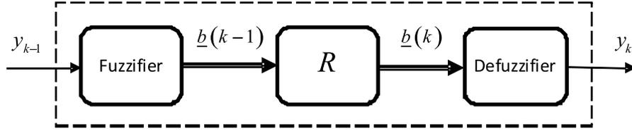
FIGURE 2. General Block Diagram of a Simple FRM
