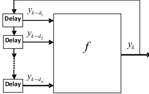
FIGURE 1. Model of a Dynamic System without any External Input
