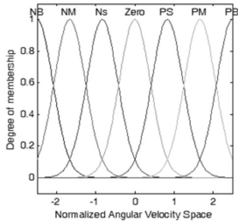
FIGURE 7. Membership Functions of Normalized Angular Velocity
