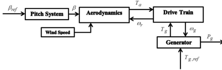
FIGURE 3. Block Diagram of the Wind Turbine Model
