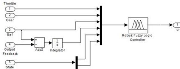
FIGURE 6. Proposed Robust Fuzzy Logic Controller for SIE Model
