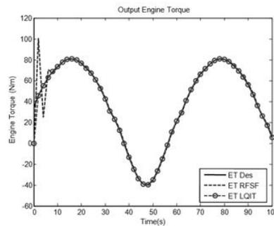
FIGURE 7. Engine Torque Produced from Application of Proposed Robust Fuzzy (ET RFSF) vs Linear Quadratic Integral Error Tracking (ET LQIT) - (gear position = 2, Throttle Input  $d(t) = 10 \sin(0.1t) + 10$ )
