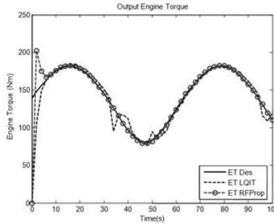
FIGURE 8. Engine Torque Produced from Application of Proposed Robust Fuzzy (RFProp) vs. Linear Quadratic Integral Error Tracking (ET LQIT) - (gear position = 2, Throttle Input  $d(t) = 10 \sin(0.1t) + 30$ )
