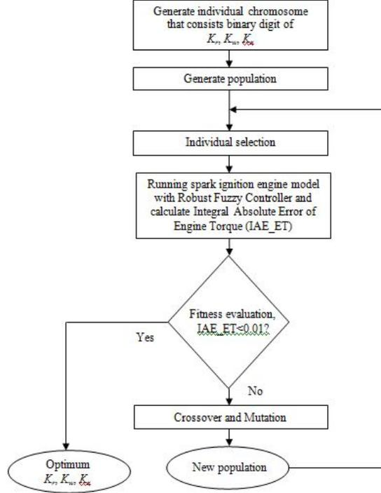
FIGURE 1. Genetic Algorithm Solution Flowchart to Optimize Gain of State Variables ( $K_x$ ), Gain of Integral Error Variables ( $K_w$ ), and Gain of Reference Signals ( $K_r$ ) of Proposed Robust Fuzzy Controller
