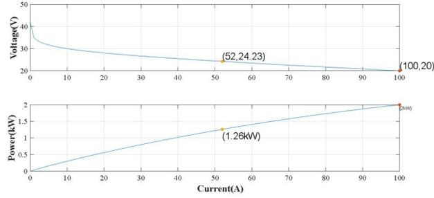
FIGURE 10. Output Voltage and Power of Selected Fuel Cell vs Load Current
