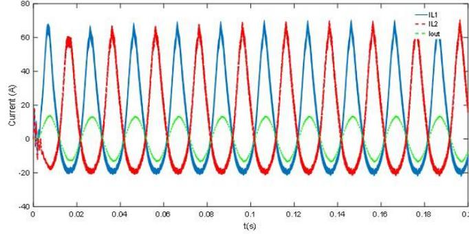
FIGURE 12. Currents of Boost Converters and Inverter
