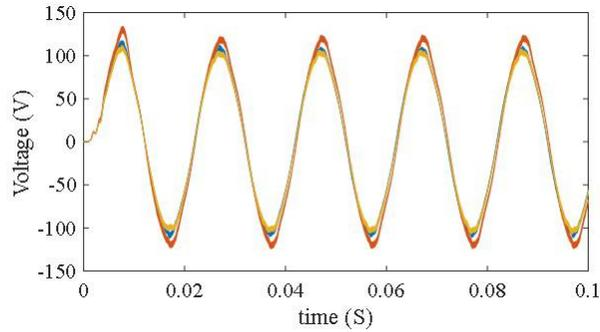
FIGURE 18. Output Voltage with Respect to Variations of  $K_I$
