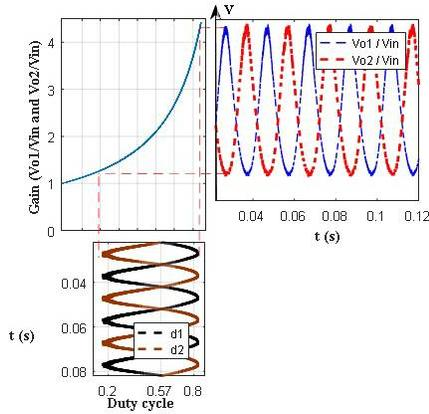
FIGURE 13. Voltages Versus Duty Cycles of Boost Converters
