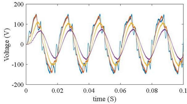
FIGURE 17. Output Voltage with Respect to Variations of  $K_P$
