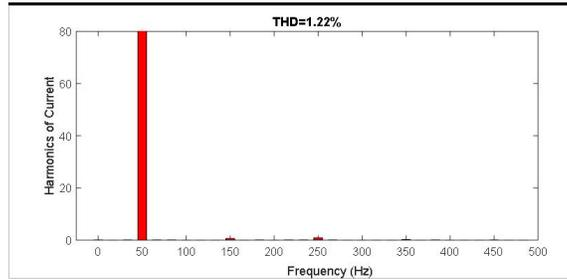
FIGURE 14. Harmonic Components of Output Current
