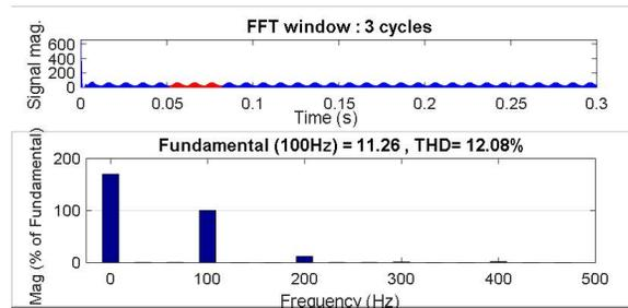
FIGURE 15. Harmonic Components of Fuel Cell Current
