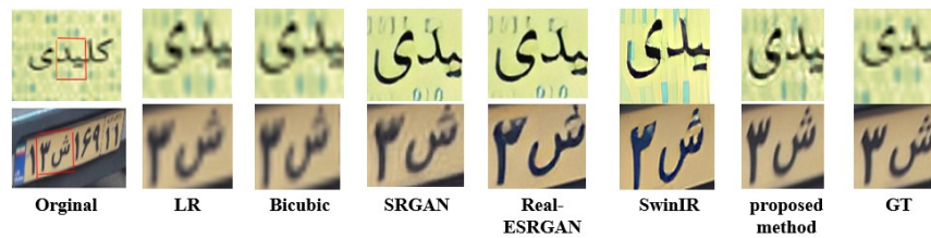
Figure 8: Visual results of FAUNet (×8). The model generates more natural and realistic textures, showing better consistency with the ground truth.
